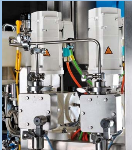
LEWA ecodos hygienic pumps with LEWA intellidrive technology (patent pending)
