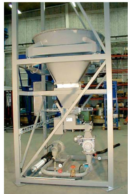
Injection of activated carbon in a flue gas channel for reduction of dioxines and mercury at Boliden Mineral copper melter at Rönnskärnsverken in northern Sweden. Turn key plant consisting of big-bag emptier, feeder, pneumatic conveying system, injection lance and controls.
