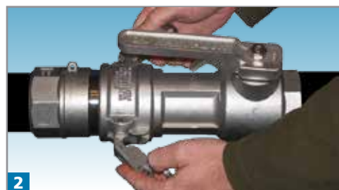
2 Cam Arms Lock Coupler and Adaptor Together
